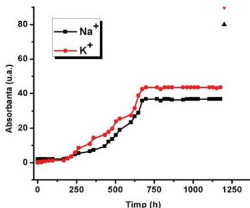
Figure 4.2: Diffusion of ions (Na<sup>+</sup> and K<sup>+</sup>) measured using a flame atomic absorption spectrometer through the pores of MCM 41 functionalized with crown ether 15C5
