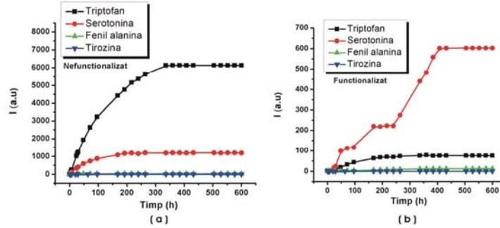
Figure 4.3: Comparison of the diffusion of amino acids (phenyl alanine, serotonin, tyrosine and tryptophan) measured by mass spectrometer coupled with liquid chromatography through the pores of MCM 41 non-functionalized (a) and functionalized with myristoyl (b)
