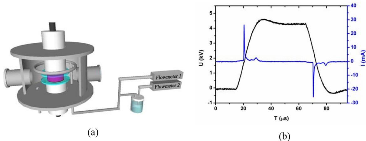
Figure 2.1. (a) Experimental set-up, (b) changes over time of the applied voltage and the current intensity through plasma
