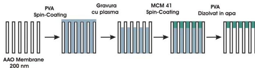
Figure 4.1: Experimental protocol used for functionalization and to obtaining the anodisc alumina membranes in order to measure the diffusion of ions ( $\text{Na}^+$  and  $\text{K}^+$ ) and amino acids (serotonin, tryptophan, tyrosine and phenyl alanine)
