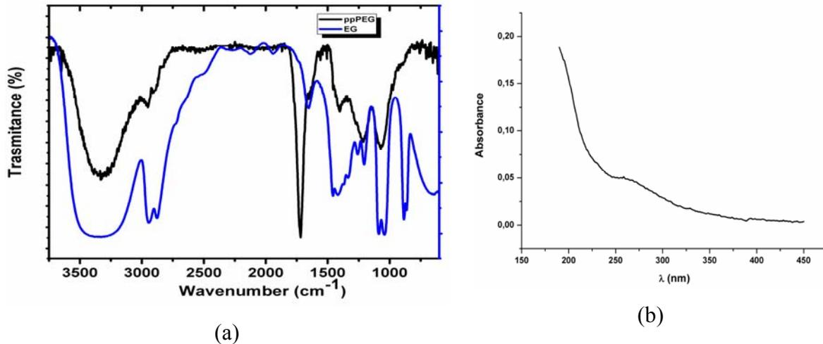
*Figure 2.2. (a) Typical FTIR spectra of ethylene glycol monomer and ppPEG obtained by APP, (b) UV spectra*
