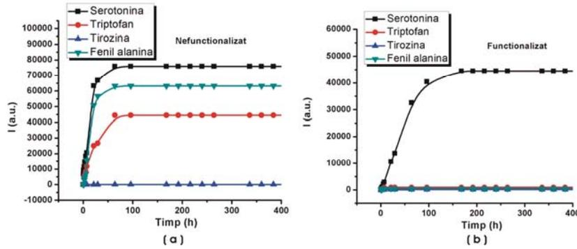
Figure 4.4 Comparison of the mixtures diffusion of amino acids (phenyl alanine, serotonin, tyrosine and tryptophan) measured by mass spectrometer coupled with liquid chromatography through the pores of MCM 41 non-functionalized (a) and functionalized with myristoyl (b)
