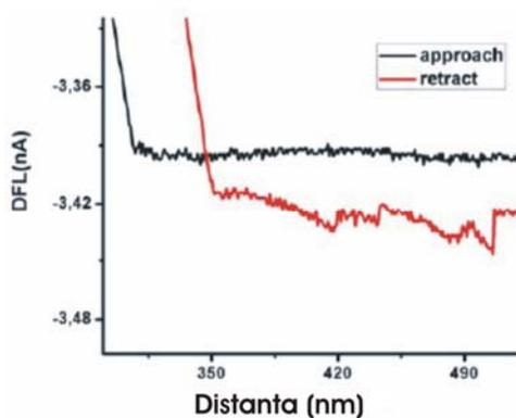
Figure 3.3. Deflection curves according to distance, in liquid medium for a tip which was 5 minutes polymerized by plasma and immersed in BSA
