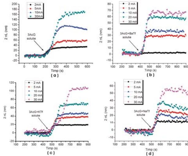
Figure 5.3. Changing in the real-time of the effective refractive index (2NL) of the silicon pores from different etching currents when introducing the 3AcG (a) 3AcG + Na + (b) 3AcG + K + (c) et 3AcG + Ba2 + (d)
