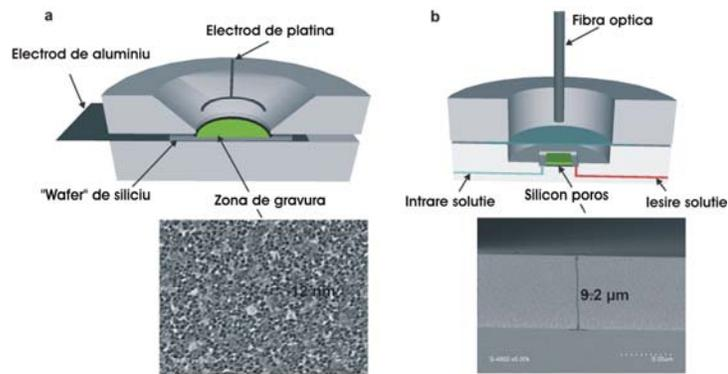
Figure 5.1. Experimental device used for obtaining the silicone pores (a) and for the quantification of the amount of molecules which pass by the interior of the porous silicon (psi) (b)
